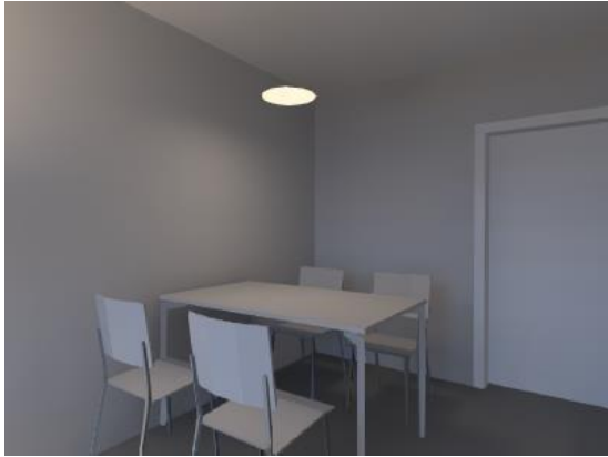
Figure 44 - Pendant placed closer towards the ceiling at 2 m.
