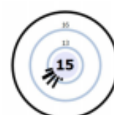
Figure 34 - UGR near bedside lamp for a person sitting at a 45-degree angle
